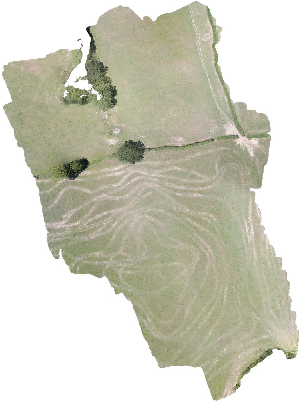
Figure 15. Composite aerial photograph taken by automatically stitching together a series of vertical images.
