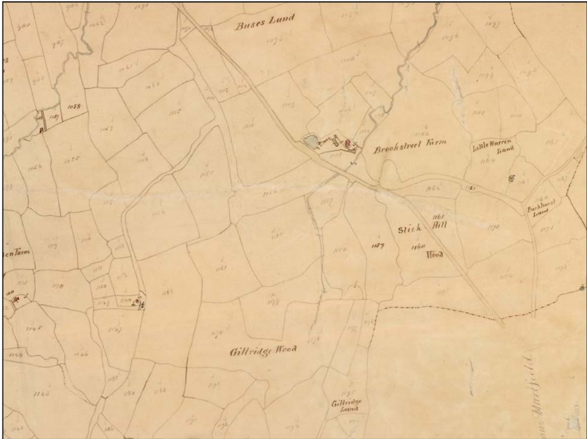
Figure 2. Example of a Tithe Map (surveyed 1844). The detail in this figure shows the same area of the parish of Edenbridge as Figure 1. Land parcels are inscribed with numbers, which relate to a book of apportionments listing the owner, extent, state of cultivation and tithe charges due. The schedule for this particular parish has been transcribed by the Kent Archaeological Society and can be accessed online ( www.kentarchaeology.org.uk ). The names of more significant woodland areas are also written in pen and ink on the map. © Kent Archives Service.
