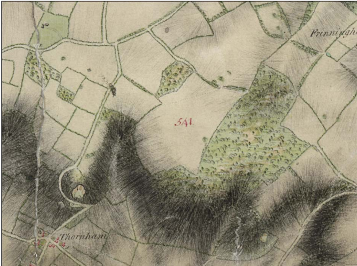
Figure 3. Example of an Ordnance Survey Drawing (1797, pen and ink on paper, produced at 6 inches to 1 mile). This employs a more generalized set of symbols to indicate trees than the later maps but the sophistication of the surveying is apparent. Note the careful attention to the depiction of relief through use of dark hachuring. This partly obscures other topographic details along the north downs escarpment but elsewhere wooded enclosures, some as small as half an acre in size, are clearly depicted. The numeral in red ink is an accurate spot height.
