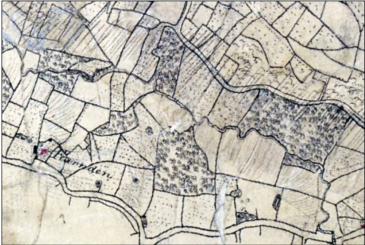
Figure 3. Example of an Ordnance Survey Drawing (produced in the field at 3inches to 1 mile in 1789). This employs a more generalized set of symbols to indicate trees but the sophistication of the surveying is clear with careful attention to the depiction of relief through cross hatching and the inclusion of small wooded enclosures.
