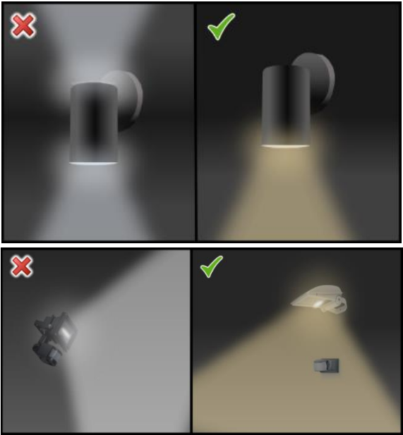
Fig 8: external lighting fittings – right hand images show directional, shielded light creating less upward skyglow.
