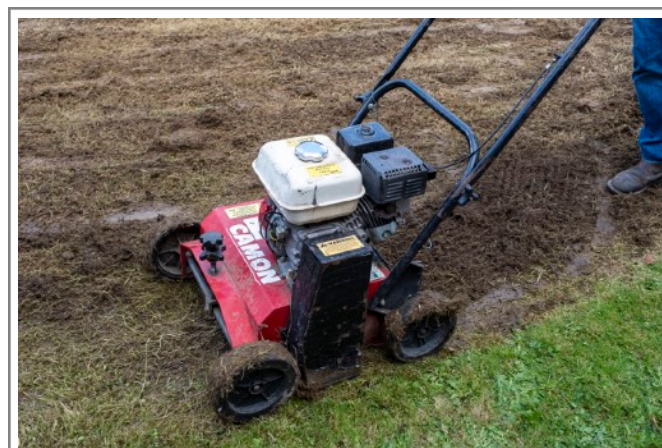
Result of Scarfing Existing Grass To Create Bare Ground Before Seeding
