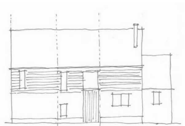
...should be used to inform the proportions and scale of proposed new buildings. The sketch shows a new building which reflects the bay divisions and opening distribution seen in traditional buildings on the farmstead
