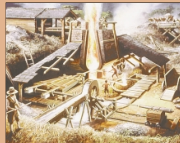
A typical Wealden, gun casting blast furnace of the 17th century. It is built against a bank to allow charcoal and ore to be tipped into the top. Furrows were shaped in the sand of the casting floor into which the molten iron was poured.
